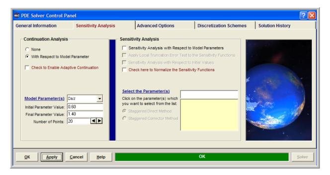
In the Continuation Analysis group click With Respect to Model Parameter and subsequently select the parameters **Dar** from the drop down list; enter the *Initial Parameter Value*, the *Final Parameter Value* and the *Number of Points* for the continuation analysis
