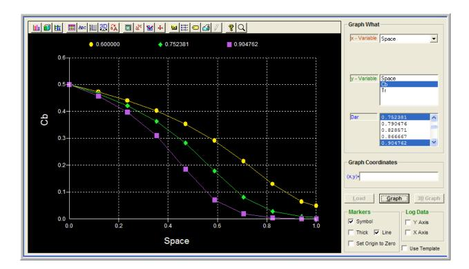
In this window fist we click **Load** to load the numerical results. Then in the **Graph What** group we select the **x-variable** (here **Space**), the **y-variable** (here concentration, **Cb**) and also a number of values of the Damköhler number; then click **Graph**. You should see the graph that appears above. You may now click on the graph toolbar and modify the type, title, symbol, the style and miscellaneous other properties of the graph.
